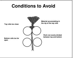
the possibility exists that material may begin to "pile up" in the nip. This condition must absolutely be avoided since the grain slipping in the roll nip will cause greatly accelerated roll wear.
