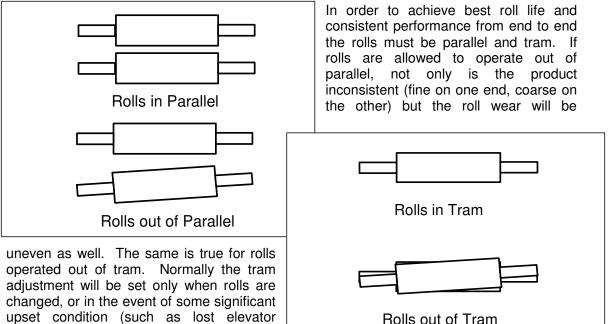
upset condition (such as lost elevator buckets and bolts appearing in the nip of the rolls).
