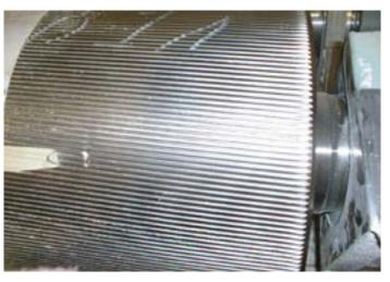
when roll adjustments are made, running the rolls together with pressure and no feed will greatly accelerate roll wear. Evidence of roll to roll contact would be corrugations with tops that appear flat, with sharp or broken edges. There will normally be some circumferential grooving or scratches in the rolls as well. Roll to roll contact is most obvious due to the noise
